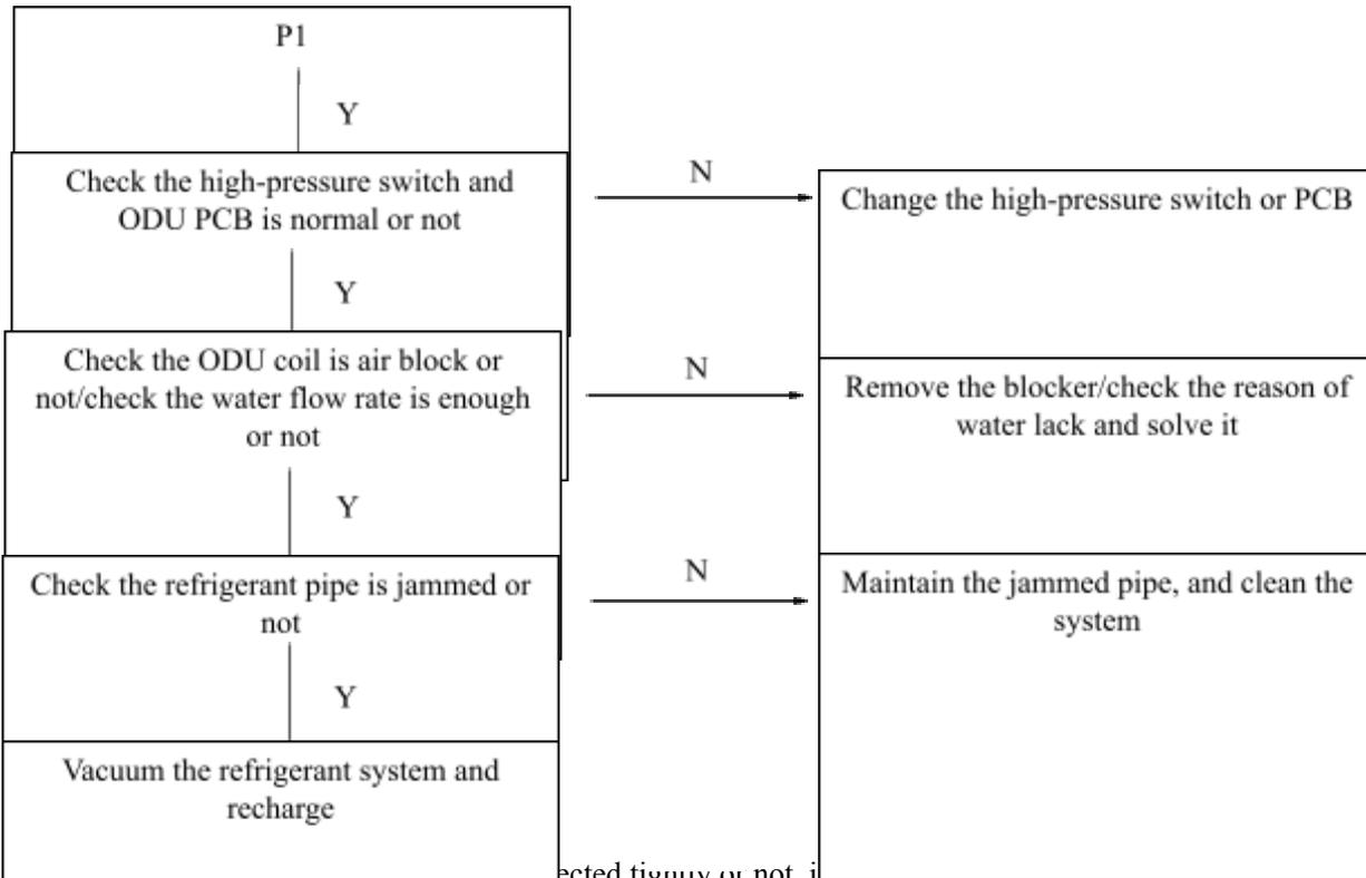
ected tightly or not, if not, connect it with controller, then wait for the refrigerant system balance, if the P1 high-pressure switch is normal. If the ODU PCB, if P1 error disappears, that means the high-pressure switch is fault, normally the resistance of the high-pressure switch is 0Ω, always close replace it.
