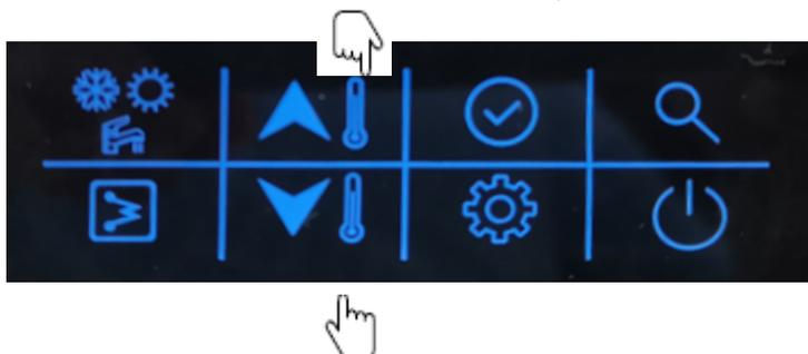
5 After hour setting, press the “confirm” button to enter minute setting, the minute is flashing at this moment.
