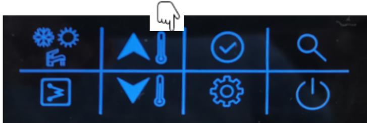
7 Press “confirm” button to confirm and exit ( ) setting. You can also press “setting” button to go to next parameter. (Refer the user parameter configuration for the full parameters setting)
