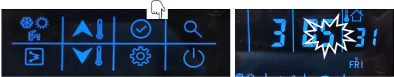
6 Then press “up” or “down” button to set the correct time in minute;
