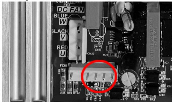
There are four ports from left to right: GND/+15V/control signal/feedback signal, if the +15V is not correct, replace the ODU PCB.
