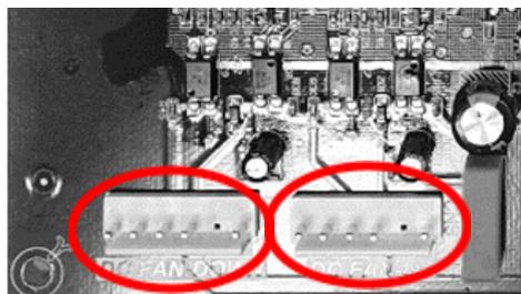
For each port, there are five ports from left to right: GND/+15V/control signal/feedback signal, if the +15V is not correct, replace the fan motor driven board.
